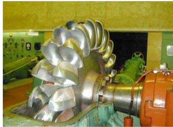
A Pelton turbine above and insert on left. A blade type turbine to the left. The pressure drop and flow rate determine which one is best for the given case.
