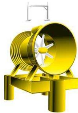
A proposed underwater tidal flow turbine farm. Each turbine is for 1 MW with a diameter of 11.5 m mounted on the seafloor.
