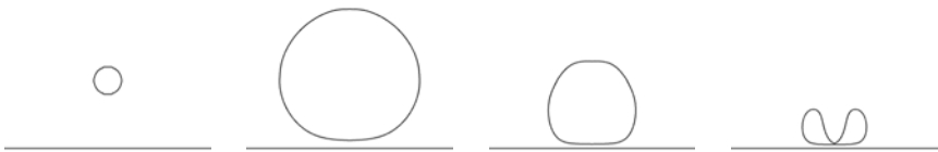
Figure 1: Jet formation through the oscillation of a bubble near a wall.
