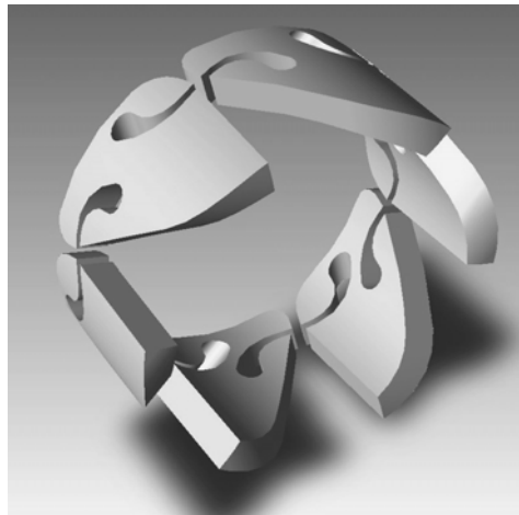
Figure 5: The stator cascade of six very thick, very short span airfoils from the previous Fig. 4. There is a control nozzle on both sides of the gap between the airfoils.
