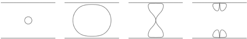
Figure 2: The jet formation through the oscillation of a bubble between a couple of parallel walls.
