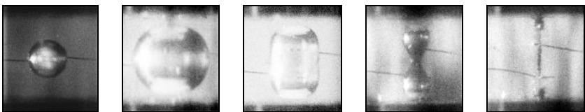
Figure 4: Experimental observation of a bubble oscillation between a couple of parallel walls, \gamma_{1,2} = 1.1 , [7].
