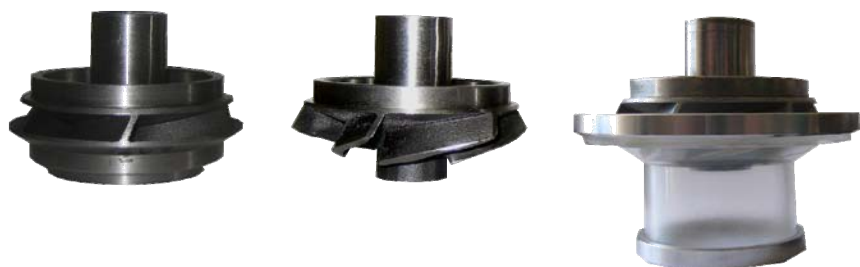
Figure 3: Impeller development process.
