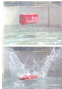
Figure 5: Impact on water of the triangular shape – V_{\text{impact}}=4.4 m/s (Politecnico Di Milano test facility).
