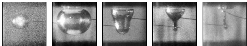
Figure 8: Experimental observation of a bubble oscillation between a couple of parallel walls, \gamma_1 = 1.3 and \gamma_2 = 0.9 , [7].
