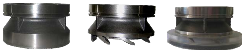
Figure 2: Top diffuser development process.
