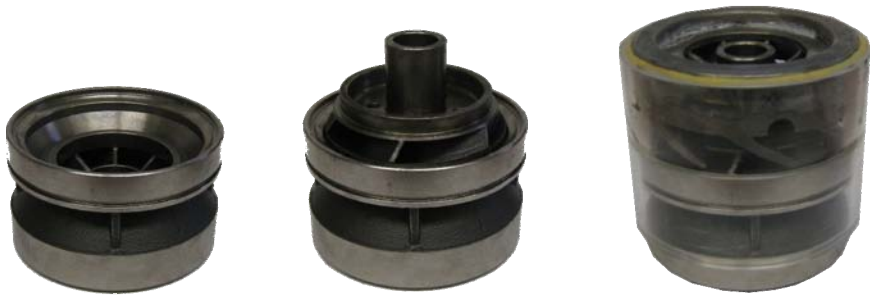
Figure 5: Entrance stage assembly process.
