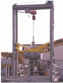
Figure 8: Impact on water of a deformable cylindrical shape – V_{\text{impact}}=10 \text{ m/s} (CIRA’s LISA test facility).
