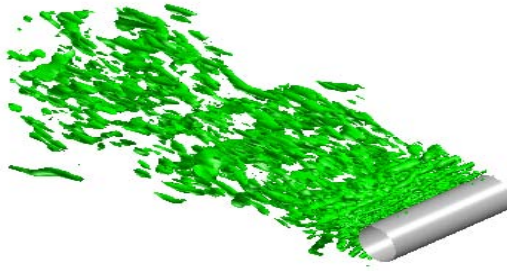
Figure 2: Iso-surfaces of Q behind cylinder for Re = 3900 .
