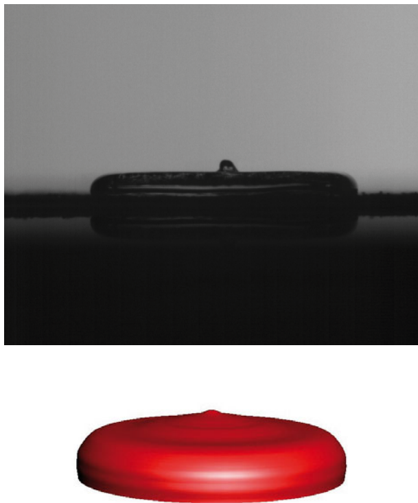
Figure 3. Comparison of the spreading phase of the cylinder impacting a rigid surface. Experiments by L. - H. Luu and Y. Forterre (2009) are shown on the top, computed results are shown on the bottom.
