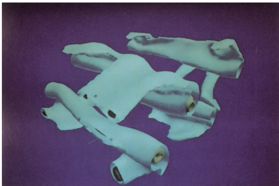
Plate 16: Same simulation as in Plate 15, showing a passive-scalar field at a later time, and the longitudinal stretching of hairpins.
