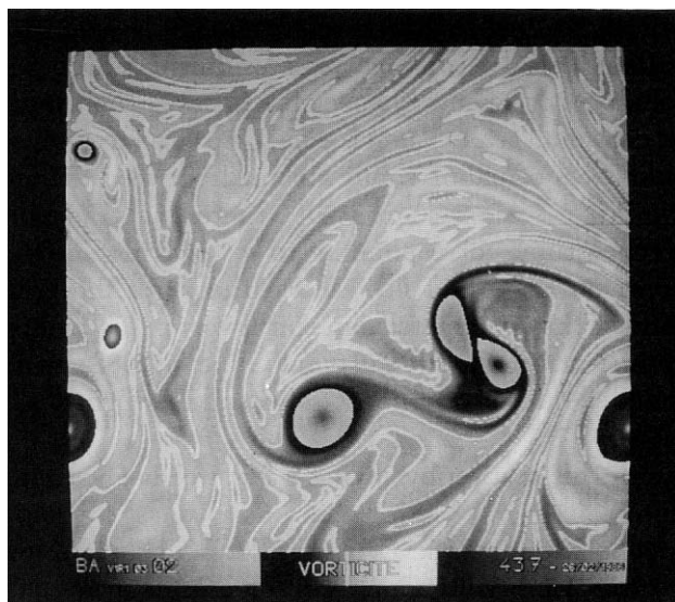
Figure 8.4. Vorticity distribution in a DNS of two-dimensional turbulence, showing in particular a pairing and a dipole (courtesy M. Farge, Paris).
