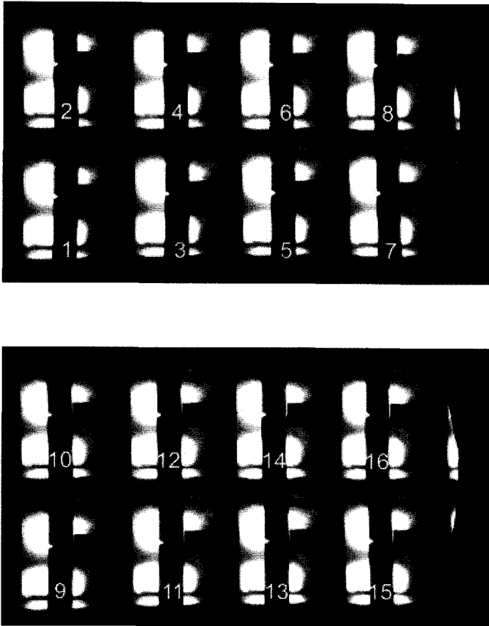
Fig. 7.2. Two separate sequences of high speed photographs in a one-point impact experiment of a Charpy specimen at room temperature. The specimen did not fracture. The rigid body kinematics is evidenced from the growing gap that develops at the specimen-bar interface. The first evidence of loss of contact appears between frames 4-5, corresponding to t = 82.5 \mu\text{s} . (Reprinted from [13]).
