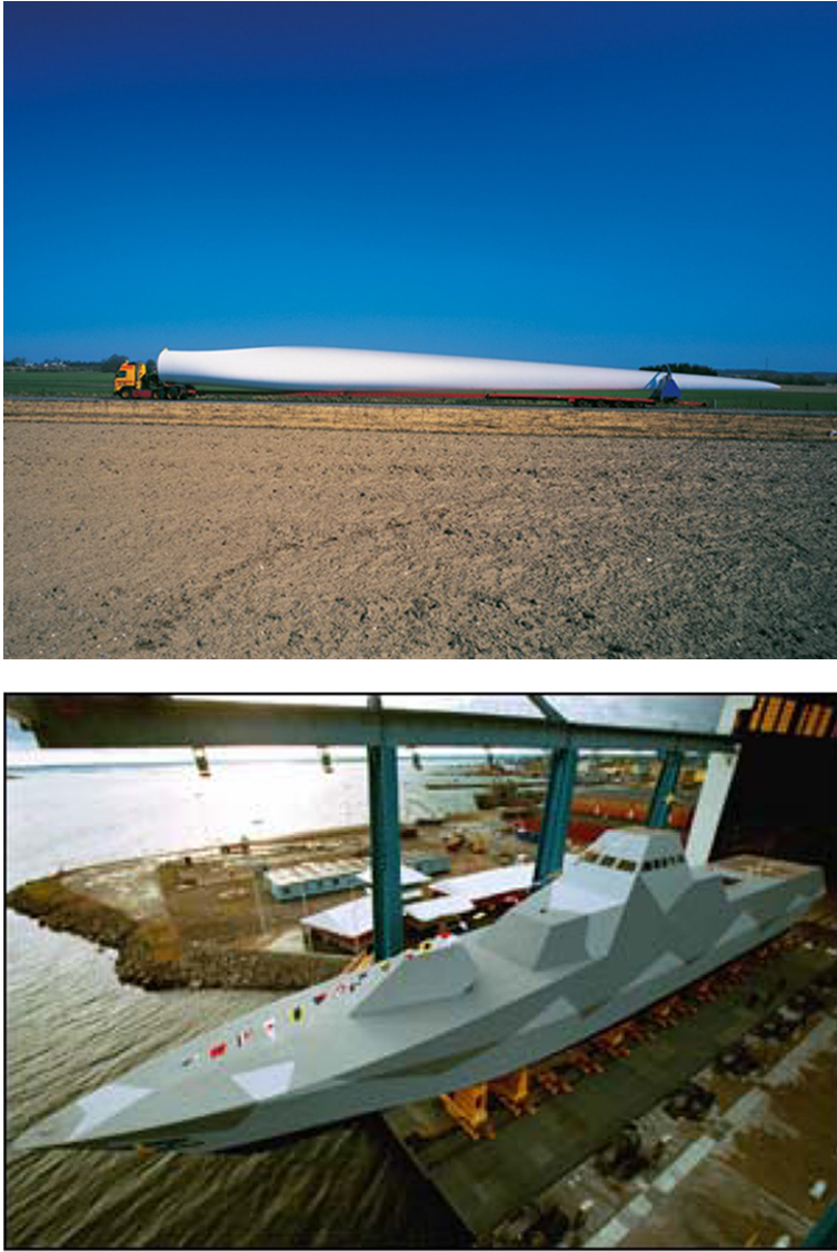
Figure 1.2 Examples of sandwich structures.
