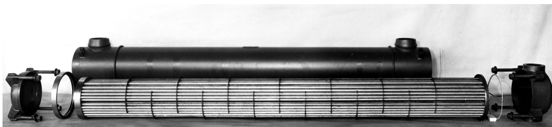
Figure 3.5 Typical commercial one-shell-pass, two-tube-pass heat exchangers.
