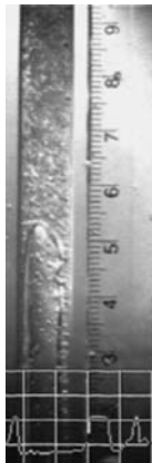
Figure 64. Flow image at 1-g for flow 11. The 1-g flow shows a similar situation where one long bubble follows the tail of another. However, this tail leaves a long trail of small dispersed bubbles in the long liquid slug
