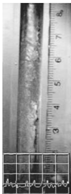
Figure 100. Flow image at 1-g for flow 17. The 1-g flow shows a much larger frothy disturbance and possibly bridging. Annular flow is present at the top of the image
