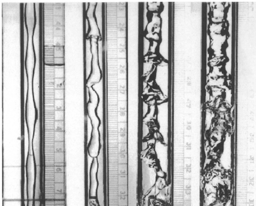
Figure 1-4. Typical images of simulated air-water inverted annular flow (It is cocurrent down flow)
