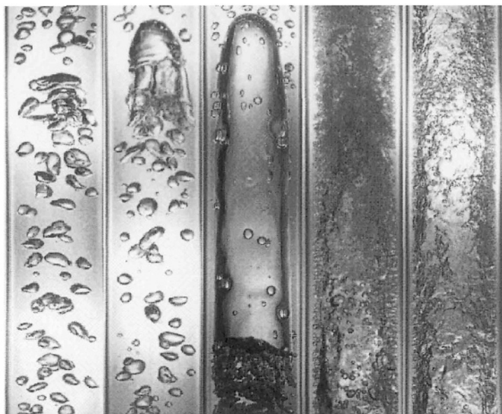
Figure 1-1. Typical air-water flow images observed in a vertical 25.4 mm diameter pipe
