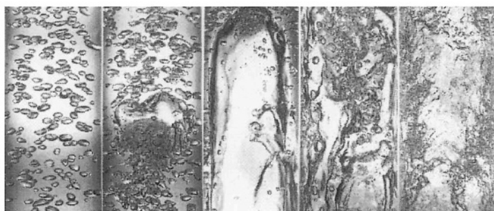
Figure 1-2. Typical air-water flow images observed in a vertical 50.8 mm diameter pipe
