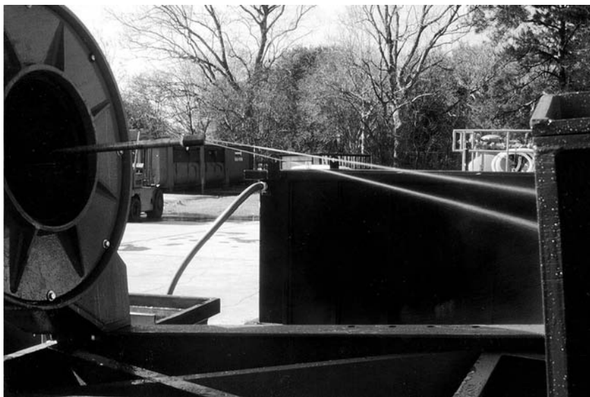
Figure 5.3. Pulsating nozzle assembly for rocket washout
