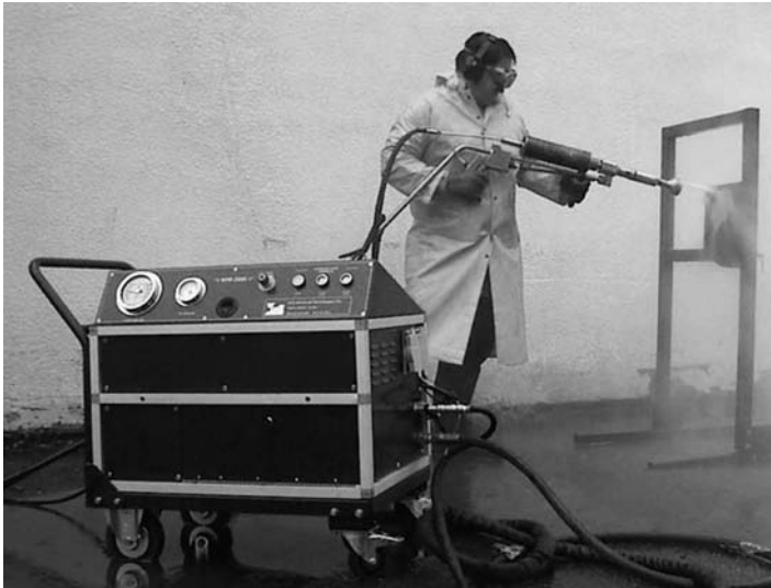
Figure 4.11. Forced pulse machine ( Courtesy of Advanced Technologies )
