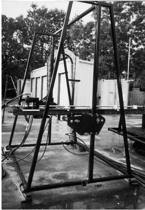
Figure 12.3. Chlorine cell cleaner nozzle lance indexer
