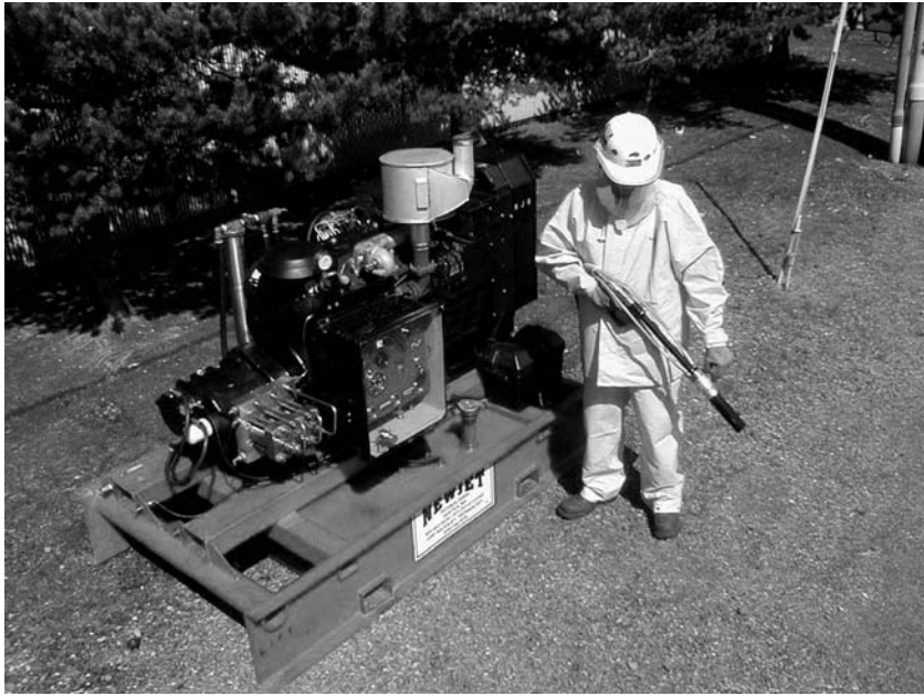
Figure 1.12. Ultra-high-pressure portable water jetting unit ( Courtesy of NewJet )
