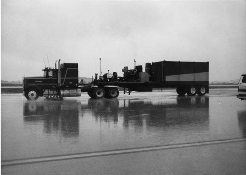
Figure 12.8. Runway cleaning equipment truck ( G. Pegoda )
