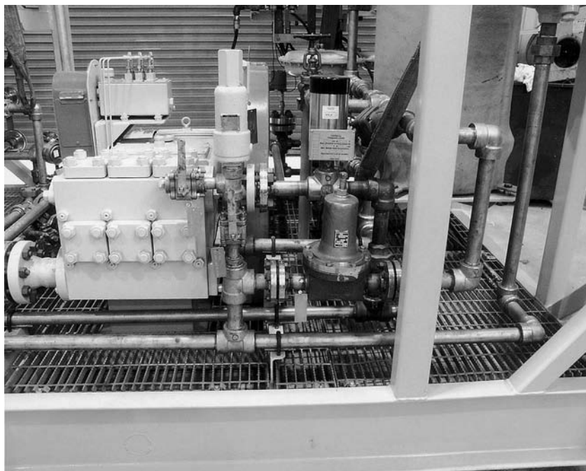
Figure 10.2. Triplex pump used in the hot water washdown unit
