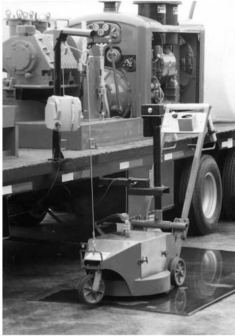
Figure 12.13. Runway cleaning lawnmower-type equipment ( Courtesy of Aqua-Dyne )
