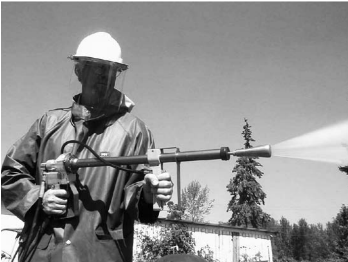
Figure 4.13. Ultra-high pressure rotary jet ( Courtesy of New Jet Technologies )
