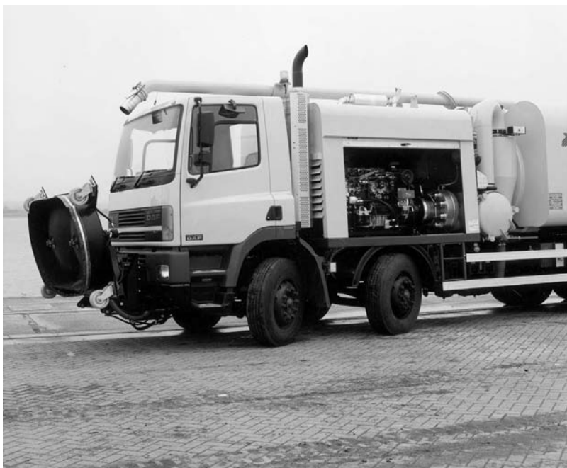
Figure 12.17. Runway cleaning truck with vacuum system ( Courtesy of Harben )
