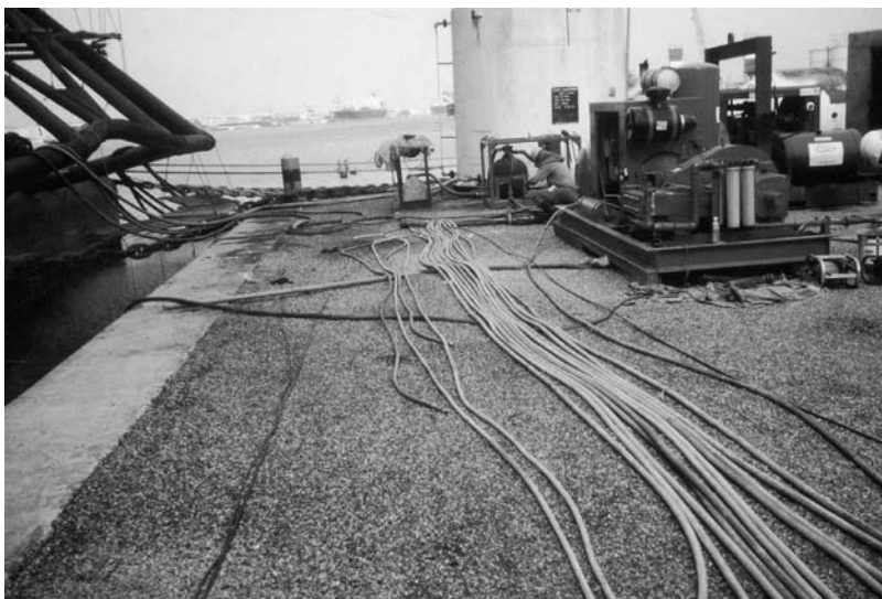
Figure 8.5. 40,000-psi hose being inspected for damage
