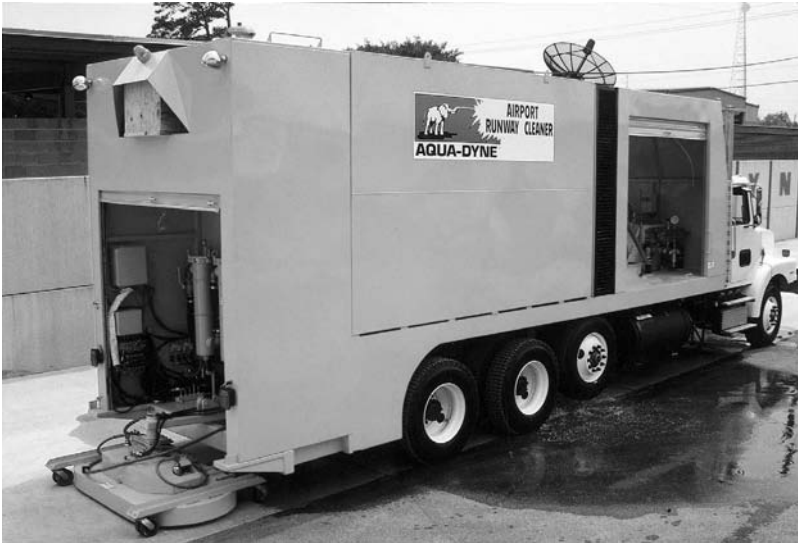
Figure 12.11. Runway cleaning equipment truck ( Courtesy of Aqua-Dyne )
