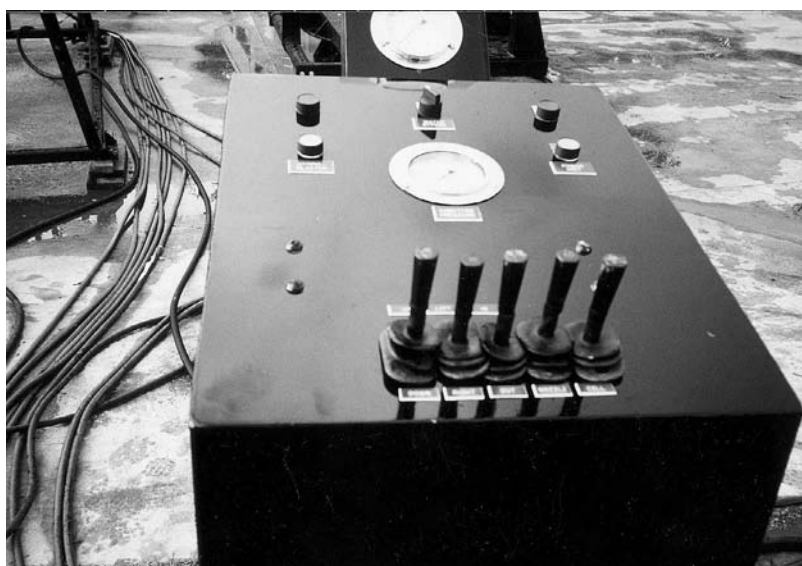
Figure 12.2. Chlorine cell cleaner system console
