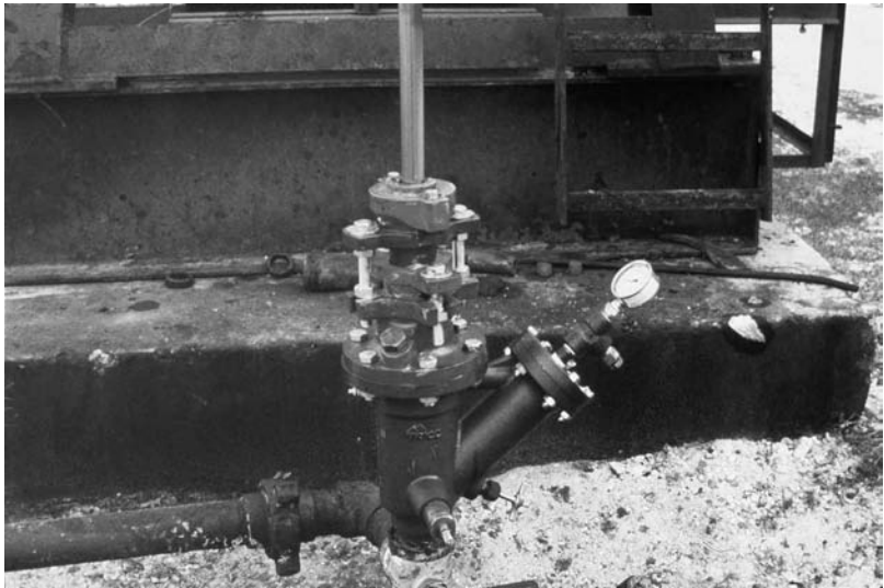
Figure 9.5. Fluid Hydro-Balanced rod pump seal (H. Palmour)
