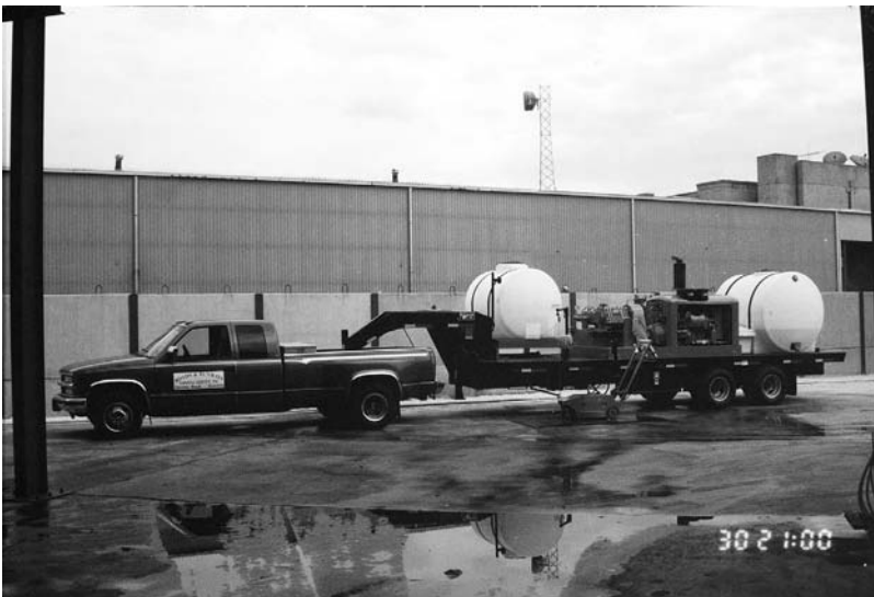
Figure 12.12. Runway cleaning equipment trailer ( Courtesy of Aqua-Dyne )
