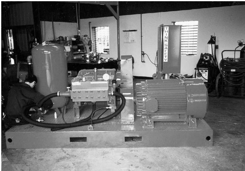
Figure 12.4. Chlorine cell cleaner 300 HP pump unit
