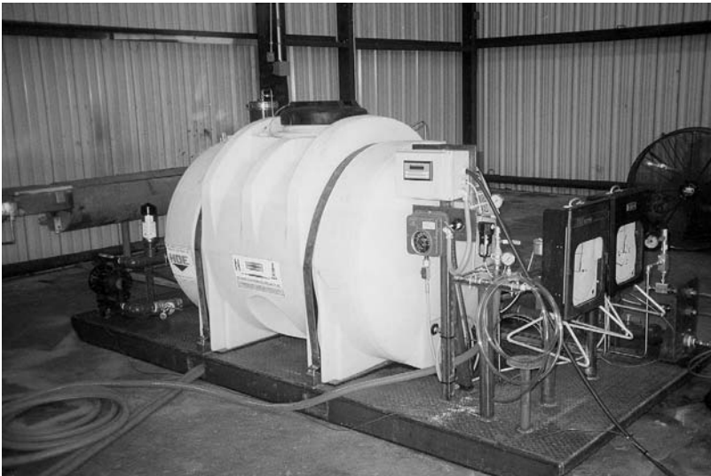
Figure 11.5. Methanol test system with supply tank and instrumentation
