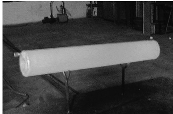
Figure 5.17 Isothermal oven for growing crystals experiments. Working fluid: sodium; dimensions: length, 500 mm; outside diameter, 51 mm; inner working space diameter 25 mm.
