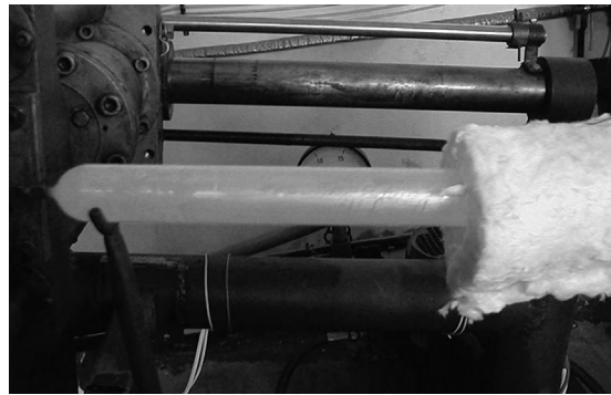
Figure 5.16 Sodium heat pipe during manufacturing process. Dimensions: length, 2800 mm; outside diameter, 38 mm; inside diameter, 32 mm; destination: catalytic reactors.
