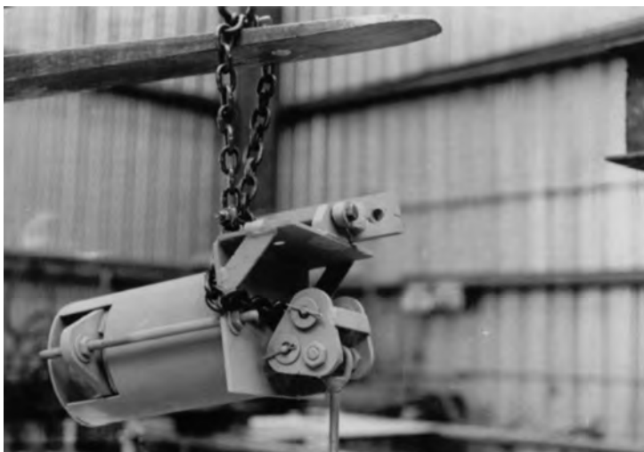
Figure 5-7b. Fabricated constant spring tested in field shop before installation.
