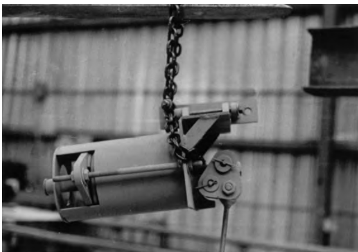
Figure 5-7a. Fabricated constant spring tested in shop.
