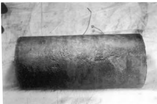
Figure 1-10. Test specimen before burst test. Courtesy of Dr. John F. Kiefner, PRCI, and the Oil and Gas Journal .
