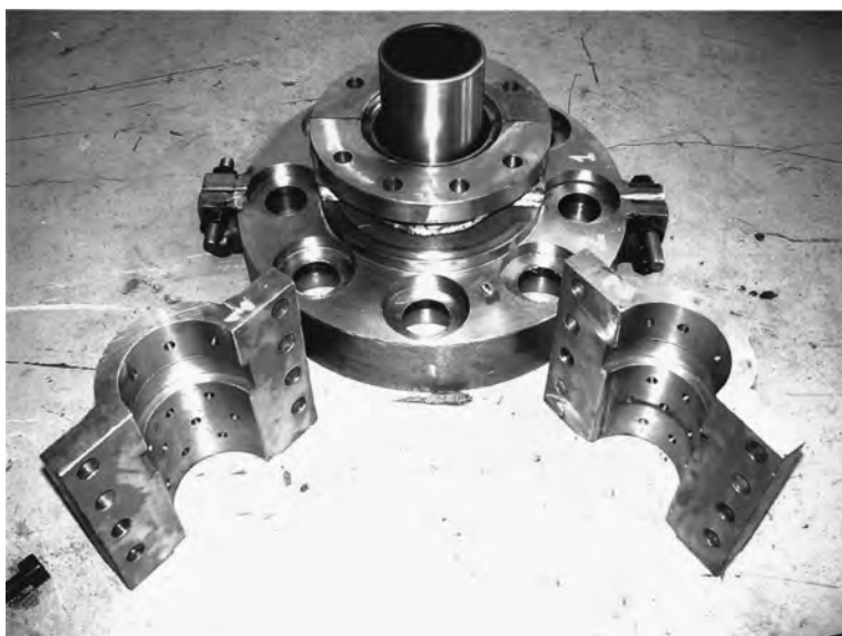
Figure 6-30b. Photo of clamp dismantled. The shear pins were installed in the holes.
