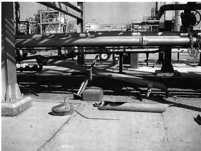
Figure 4-7a. View of a nitrogen gas line accidentally loaded with liquid nitrogen.
